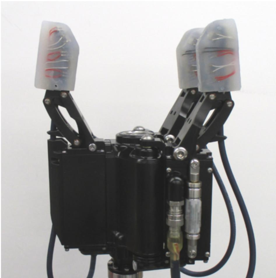
During lab testing, the STARFISH prototype used three tactile-sensing fingers to successfully achieve a variety of fine- and large-gripping skills, including squeezing a pair of tweezers and grasping larger objects. Each finger conforms to the shape it is grasping, enabling it to securely hold objects upon contact.
